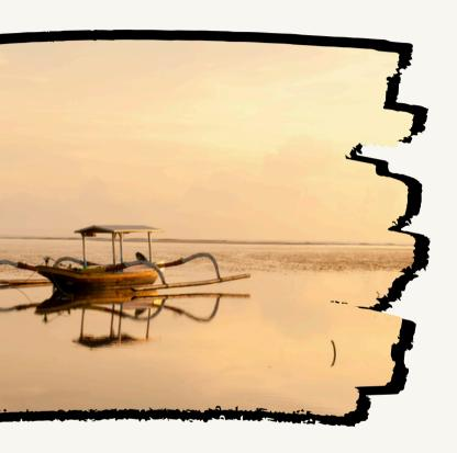
A jukung is a traditional Indonesian boat. It looks like an ordinary canoe — it is long and narrow and often made of wood. On each side of the boat are long floats called outriggers. The outriggers help the boat keep its balance on the water and not tip over. In the back of the jukung is a powerful outboard engine that propels the boat forward
